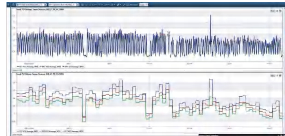
PST and PLT value curve with SVC compensation during EAF production
