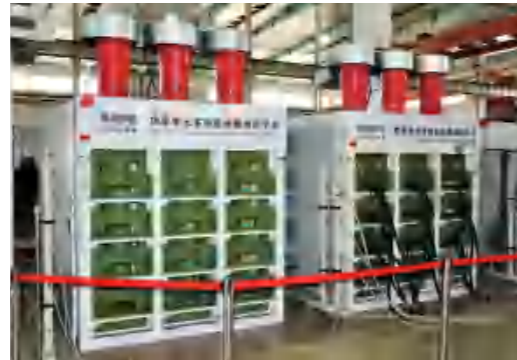
Full load and multifunctional test platform for power modules (1.1 times overload)
