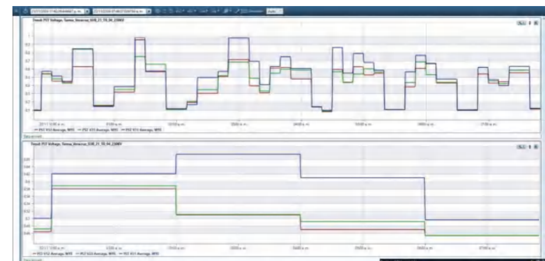
PST and PLT value curve with STATCOM compensation during EAF production
