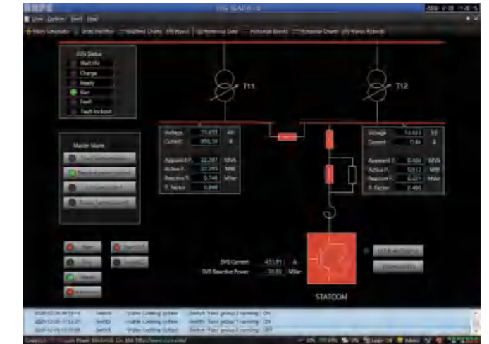
Main interface of equipment operation (after compensation)
