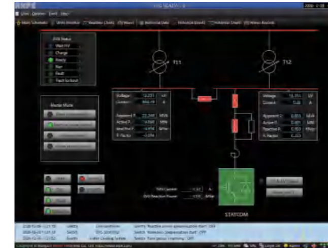
Main interface of equipment operation (before compensation)
